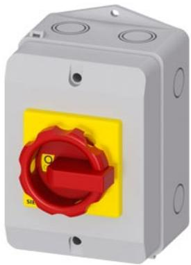
SENTRON, Switch disconnector 3LD, emergency switching-off switch, 3- pole, Iu: 32 A, operating power / at AC-23 A 400 V: 11.5 kW, molded-plastic encapsulation for metric cable gland, rotary operating mechanism, red/yellow
