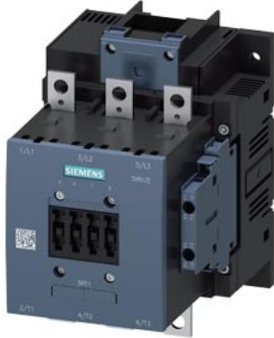
power contactor AC-1 275 A / 690 V / 40 °C 3-pole, Uc: 220-240 V AC(50-60 Hz) / DC drive: conventional auxiliary contacts 2 NO + 2 NC main circuit: busbar control and auxiliary circuit: screw terminal
