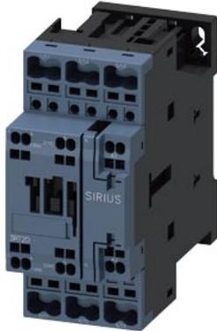
power contactor, AC-3e/AC-3, 12 A, 5.5 kW / 400 V, 3-pole, 110 V AC, 50/60 Hz, auxiliary contacts: 1 NO + 1 NC, spring-loaded terminal, size: S0
