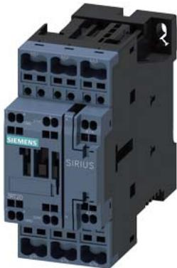
power contactor, AC-3e/AC-3, 12 A, 5.5 kW / 400 V, 3-pole, 24 V DC,
