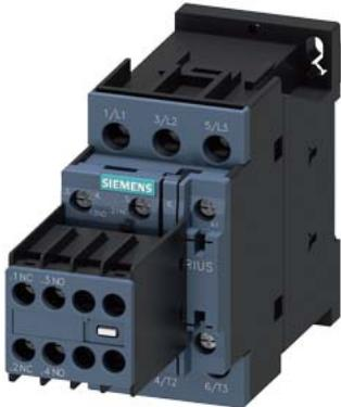
power contactor, AC-3e/AC-3, 12 A, 5.5 kW / 400 V, 3-pole, 230 V AC, 50 Hz, auxiliary contacts: 2 NO + 2 NC, screw terminal, removable auxiliary switch
