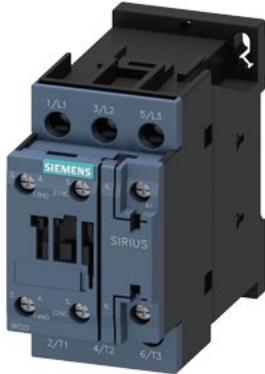
power contactor, AC-3e/AC-3, 32 A, 15 kW / 400 V, 3-pole, 110 V AC, 50 Hz, auxiliary contacts: 1 NO + 1 NC, screw terminal, size: S0
