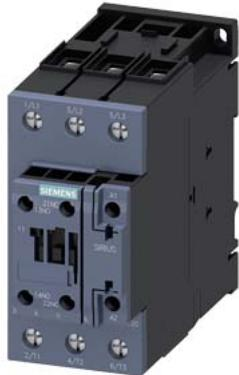
power contactor, AC-3e/AC-3, 41 A, 18.5 kW / 400 V, 3-pole, 110 V AC, 50 Hz, auxiliary contacts: 1 NO + 1 NC, screw terminal
