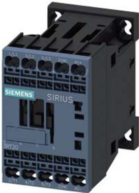
power contactor, AC-3e/AC-3, 7 A, 3 kW / 400 V, 3-pole, 24 V DC, 0.7-1.25\* Us, with integrated suppressor diode, auxiliary contacts: 1 NC, spring-loaded terminal, size: S00, suitable for PLC outputs, not expandable with auxiliary switch
