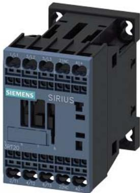
power contactor, AC-3e/AC-3, 7 A, 3 kW / 400 V, 3-pole, 24 V DC, auxiliary contacts: 1 NC, spring-loaded terminal
