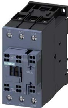
power contactor, AC-3e/AC-3, 80 A, 37 kW / 400 V, 3-pole, 230 V AC, 50 Hz, auxiliary contacts: 1 NO + 1 NC, main circuit: screw terminal, control and auxiliary circuit: spring-loaded terminal, size: S2
