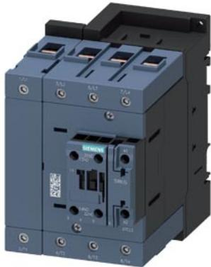
contactor AC-1, 140 A, 400 V / 40 °C, 4-pole, 20-33 V AC/DC, 50/60 Hz, with integrated varistor, auxiliary contacts: 1 NO + 1 NC, screw terminal, size: S3
