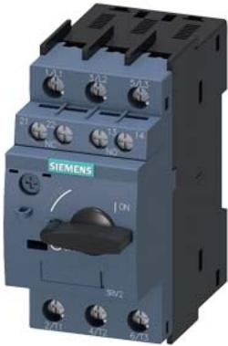
Circuit breaker size S00 for motor protection, CLASS 10 A-release 10...16 A N-release 208 A screw terminal Standard switching capacity with transverse auxiliary switches 1 NO+1 NC
