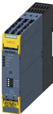
SIRIUS safety relay Basic unit Advanced series with time delay 0.5-30 s electronic enabling circuits 2 NO instantaneous 2 NO delayed Us = 24 V DC screw terminal
