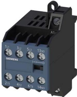
power relay, AC-3e/AC-3, 8.4 A, 4 kW / 400 V, 3-pole, 230 V AC, 45-450 Hz, auxiliary contacts: 1 NO, screw terminal
