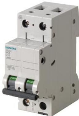
Miniature circuit breaker 400 V 6kA, 2-pole, C, 10 A
