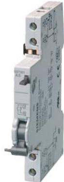
Auxiliary current switch with test button, 2 NC for circuit breaker 5SL, 5SY, 5SP Incorporated switch 5TL1, RCBO 5SU1, FI 5SV (for 5SU1 handle coupler 5ST3805-1 is required)
