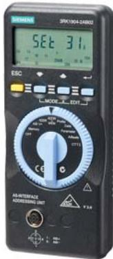
AS-Interface Addressing unit V3.0 for setting the addresses of AS-i slave modules Input/output test and further functions AS-i specification V3.0 M12 connection socket with addressing cable 1.5 m (M12 connector/hollow plug) with batteries (4 x 1.5 V LR6)
