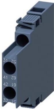
auxiliary switch, lateral, 2 NC, on the left: 51/52, 61/62, on the right: 31/32, 41/42, current path: 1 NC, 1 NC, screw terminal, for contactors 3RT2 and contactor relays 3RH2
