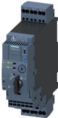
SIRIUS Compact load feeder DOL starter 690 V 24 V AC/DC 50...60 Hz 0.32...1.25 A IP20 Connection main circuit: Spring-type terminal Connection auxiliary circuit: Spring-type terminal
