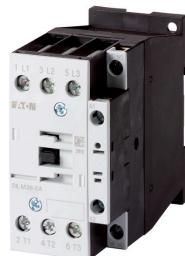
Contactor, 3 pole, 380 V 400 V 18.5 kW, 1 N/O, 230 V 50 Hz, 240 V 60 Hz, AC operation, Screw terminals
