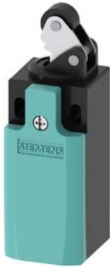
Position switch Plastic enclosure according to EN 50047, 31 mm Device connection 1 x (M20 x 1.5) 1 NO/1 NC quick action contacts integrated (not replaceable) Roller lever with plastic roller 13 mm
