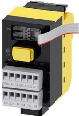
SIRIUS ACT with PROFINET: fail-safe interface module with 4 DI, 1 DQ (24 V DC), 1 AI (12-bit A/D resolution), 24 V DC, screw terminal, front plate mounting, 1 to 20 terminal modules connectable
