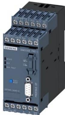
Basic unit SIMOCODE pro C, PROFIBUS DP interface 12 Mbit/s, RS 485, 4I/3O freely parameterizable, Us: 110...240 V AC/DC, input for thermistor connection Monostable relay outputs
