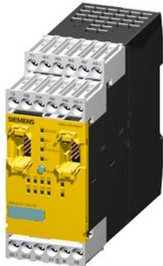
SIRIUS, Central unit 3RK3 Advanced for modular Safety system 3RK3 4/8 F-DI, 1F-RO, 1 F-DO, 24 V DC Monitoring of ASI slaves Control of 12 safe outputs on AS-Interface bus parameterizable using software Safety ES 45 mm width screw terminal Up to SIL3 (IEC 61508) Up to Performance Level E (ISO 13849-1) 9 extension modules connectable
