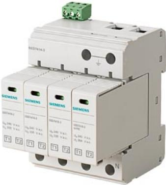
Lightning conductor T1/T2, UN 240/400 V, UC 335/264 V A.C., pluggable protective modules, 3+1 circuit (TN-S, TT), Width 72 mm with remote signaling
