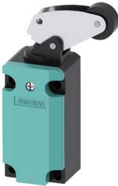
Position switch Metal enclosure 40 mm according to EN 50041 Device connection 1x (M20 x 1.5) 1 NO/1 NC quick action contacts Angular roller lever, metal lever and plastic roller 22 mm
