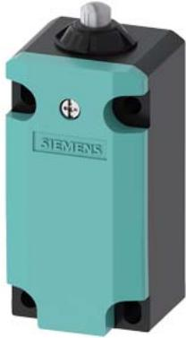
Position switch Metal enclosure 40 mm according to EN 50041 Device connection 1x (M20 x 1.5) 1 NO/1 NC slow-action contacts Plain plunger, stainless steel
