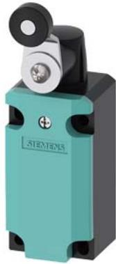
Position switch Metal with twist lever 40 mm, according to EN 50041 Increased corrosion protection 1 NO/2 NC quick action contacts functional at -40 °C Shock and vibration test according to EN 61373, Category 1B
