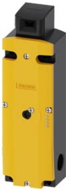
Safety position switch with tumbler Locking force 1300 N 5 directions of approaches Spring-locked Auxiliary release on front Magnet voltage 24 V DC Monitoring actuator 2 NC/1 NO Monitoring magnet 2 NC/1 NO LED display yellow/green Supplied without actuator. Actuator 3SE5000-0AV. please order separately
