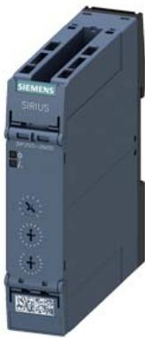
Timing relay, Multifunction 2 change-over contacts, 27 functions 7 time ranges (0.05 s...100 h) 12-240 V AC/DC at 50/60 Hz AC with LED Spring-type terminal (push-in)
