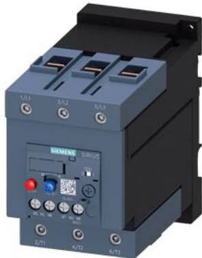
Overload relay 70...90 A Thermal For motor protection Size S3, Class 10
