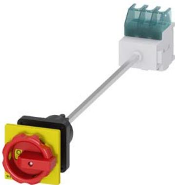
SENTRON, Switch disconnector 3LD, emergency switching-off switch, 3- pole, Iu: 25 A, operating power / at AC-23 A 400 V: 9.5 kW, floor mounting with door coupling, rotary operating mechanism, Red / yellow, central mounting 22.5 mm of the handle
