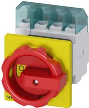
SENTRON, Switch disconnector 3LD, emergency switching-off switch, 4- pole, Iu: 32 A, operating power / at AC-23 A 400 V: 11.5 kW, front-mounted, rotary operating mechanism, Red / yellow, central mounting 22.5 mm of the handle
