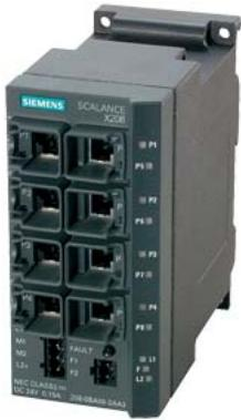
SCALANCE X208, managed IE switch, 8x 10/100 Mbit/s RJ45 ports, LED diagnostics, error-signaling contact with set pushbutton, redundant power supply, PROFINET IO device, network management, redundancy manager integrated, incl. electron. manual on CD-ROM, C-PLUG optional.
