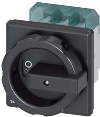
SENTRON, Switch disconnector 3LD, main switch, 3-pole, Iu: 63 A, Operating power / at AC-23 A at 400 V: 22 kW, front-mounted, rotary operating mechanism, black, 4-hole mounting of the handle
