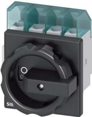
SENTRON, Switch disconnector 3LD, main switch, 4-pole,  $I_{u}$ : 32 A, Operating power / at AC-23 A at 400 V: 11.5 kW, front-mounted, rotary operating mechanism, black, 4-hole mounting of the handle
