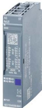
SIMATIC ET 200SP, Analog output module, AQ 4XU/I Standard, suitable for BU type A0, A1, Color code CC00, Module diagnostics, 16 bit, +/-0.3%
