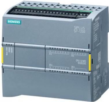
SIMATIC S7-1200F, CPU 1214 FC, compact CPU, DC/DC/relay, onboard I/O: 14 DI 24 V DC; 10 DO relay 2 A; 2 AI 0-10 V DC, Power supply: DC 20.4-28.8V DC, Program/data memory 125 KB
