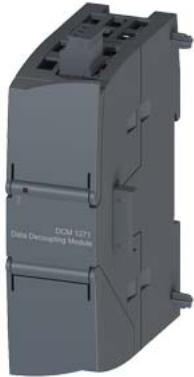
SIMATIC S7-1200, DCM 1271 Data decoupling module for AS-i Master CM 1243-2 IN: 24 V / 30 V DC OUT: 1x AS-Interface, 4 A Integrated overload protection integr. ground fault detection Signaling contact
