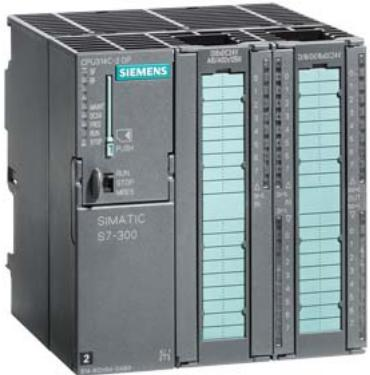
SIMATIC S7-300, CPU 314C-2 DP Compact CPU with MPI, 24 DI/16 DO, 4 AI, 2 AO, 1 Pt100, 4 high-speed counters (60 kHz), integrated DP interface, Integr. power supply 24 V DC, work memory 192 KB, Front connector (2x 40-pole) and Micro Memory Card required
