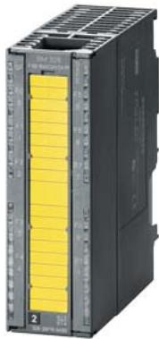
SIMATIC S7, digital output SM 326, F-DO10x 24 V DC/2A PP, fail-safe digital output for SIMATIC S7F systems, with diagnostic alarm, LVV, up to Category 4 (EN 954-1)/ SIL3 (IEC61508)/PLE (ISO13849), 1x 40-pole
