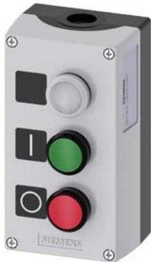
Enclosure for command devices, 22 mm, round, Enclosure material plastic, enclosure top part gray, 3 control points plastic, C=Indicator light clear, label LED 24 V, screw terminal, B=Pushbutton green, label: I, 1 NO, screw terminal, A=Pushbutton red, label: O, 1 NC, screw terminal, floor mounting, 1xM20 each on top and bottom, Labels enclosed
