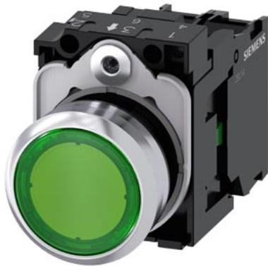
Illuminated pushbutton, 22 mm, round, metal, shiny, green, pushbutton, flat, momentary contact type, with holder, 1 NO, LED module with integrated LED 230 V AC, screw terminal
