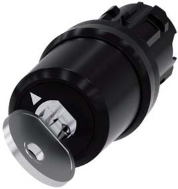
key-operated switch Siemens, 22 mm, round, plastic, lock number SSG10, with 2 keys, 2 switch positions O-I, latching, actuating angle 90°, 10:30h/13:30h, key removal O+I
