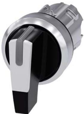
Selector switch, illuminable, 22 mm, round, metal, shiny, white, selector switch, long, 3 switch positions I>O<II, momentary contact type, actuating angle 2x45°, 10:30h/12h/13:30h
