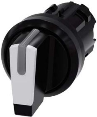
Selector switch, illuminable, 22 mm, round, plastic, white, selector switch, short, 3 switch positions I>O<II, momentary contact type, actuating angle 2x45°, 10:30h/12h/13:30h
