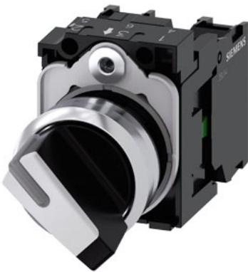
Selector switch, illuminable, 22 mm, round, metal, shiny, white, selector switch, short, 2 switch positions O-I, latching, actuating angle 90°, 10:30h/13:30h, with holder, 1 NO, 1 NC, screw terminal
