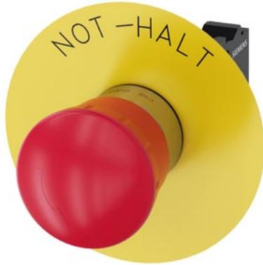
EMERGENCY STOP mushroom-type actuator, 22 mm, round, metal, shiny, red, 40 mm, positive latching, according to EN ISO 13850, rotate-to-unlatch, with yellow backing plate, inscription: NOT-HALT, with holder, 1 NC, 1 NC, spring-type terminal
