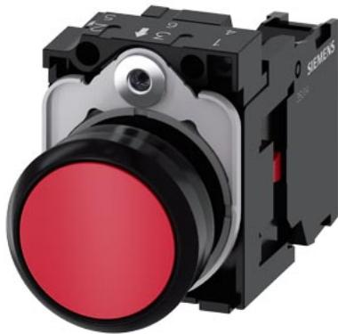
Pushbutton, 22 mm, round, plastic, red, pushbutton, flat, momentary contact type, with holder 1 NC, screw terminal
