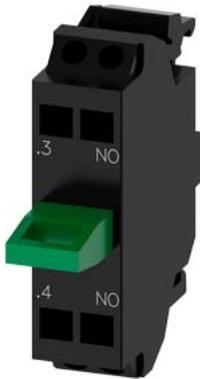
Contact module with 1 contact element, 1 NO, spring-type terminal, for floor mounting, Minimum order quantity 5 or a multiple thereof
